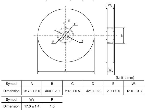
Dimensions of reel (Material : Polystyrene) CGA1, CGA2, CGA3, CGA4, CGA5, CGA6
