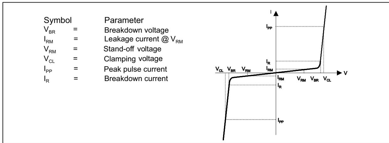
Table 2. Electrical characteristics (values,  $T_{amb} = 25\text{ °C}$ )
