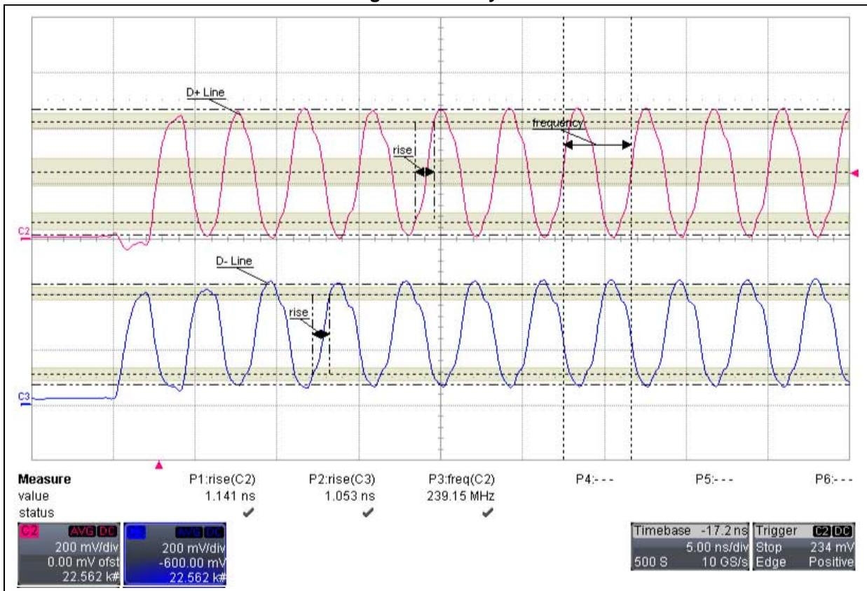
Figure 18. Total harmonic distortion on differential lanes
