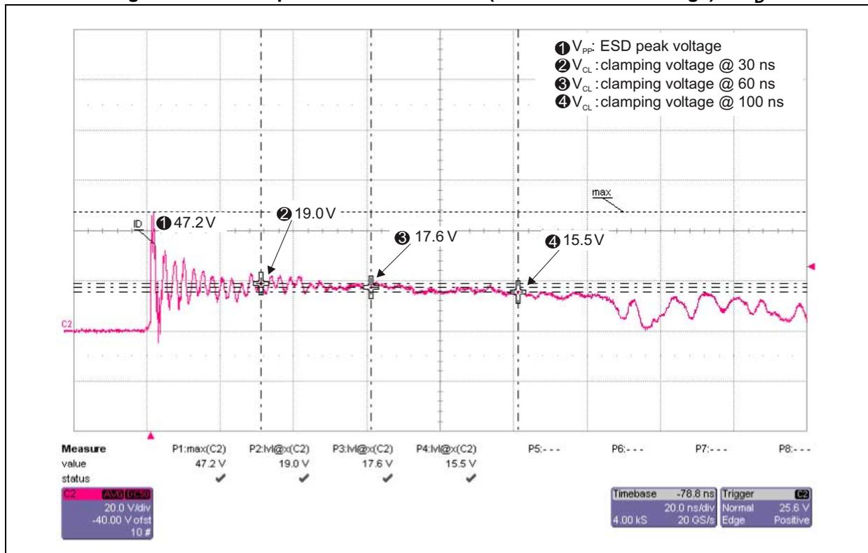
Figure 11. ESD response to IEC 61000-4-2 (-8 kV contact discharge) on I<sub>D</sub>
