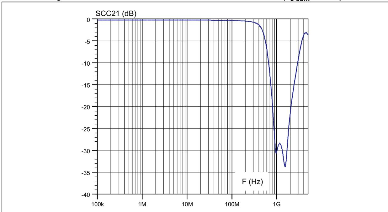
Figure 5. ID frequency response measurement ( $Z_0 = 75 \Omega$ )
