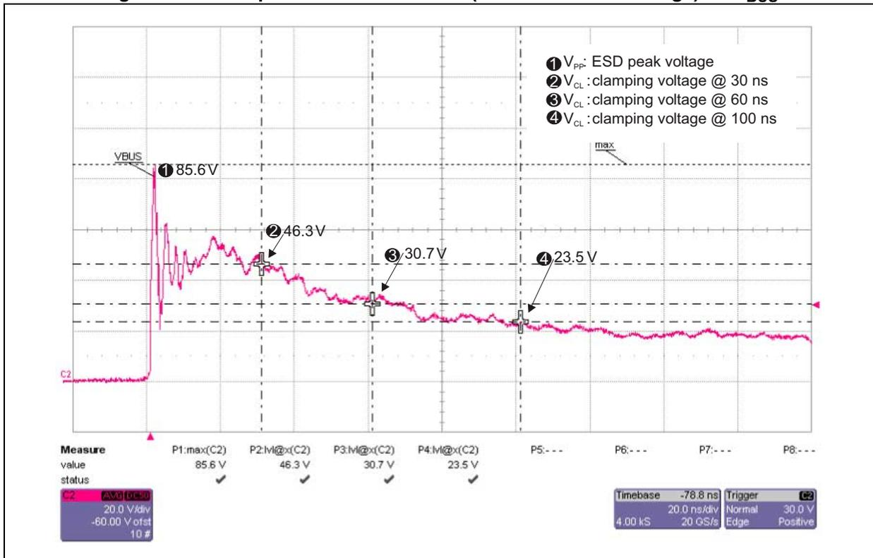
Figure 9. ESD response to IEC 61000-4-2 (-8 kV contact discharge) on V<sub>BUS</sub>
