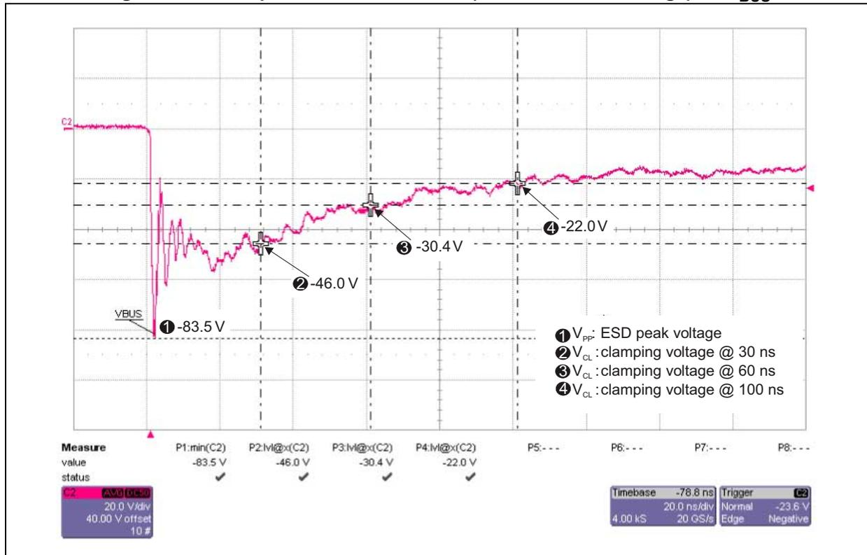
Figure 10. ESD response to IEC 61000-4-2 (+8 kV contact discharge) on I<sub>D</sub>
